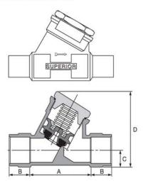
Type 802B Check Valve Series ODS x ODS Tube Extensions\*
